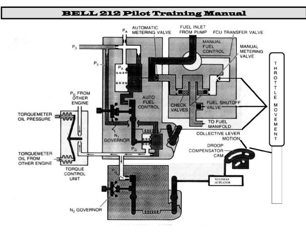
FIGURE 7-39 Fuel Control Automatic Mode
