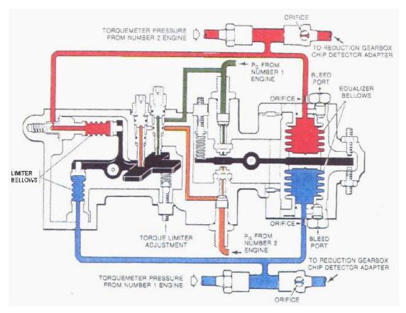
Figure 7-42 Torque Control Unit Diagram
