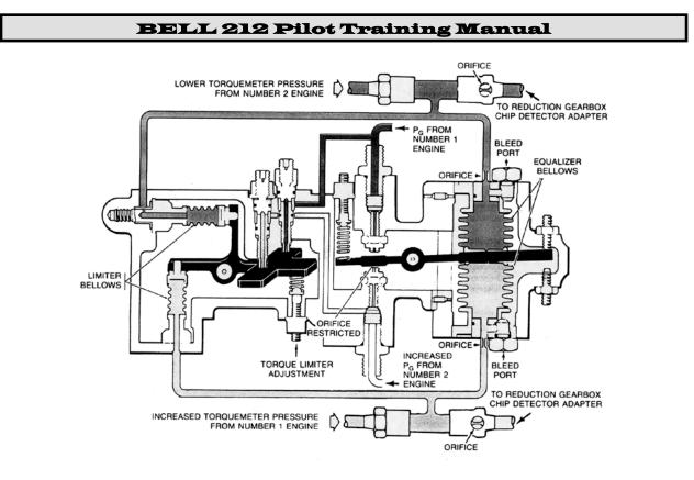
Figure 7-43 No. 1 Engine Torque Higher that No. 2 Engine Torque
