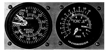
HIGH-SIDE FCU FAILURE DURING LOW POWER DEMAND
