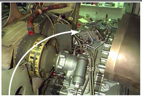
Figure 7-41 Torque Control Unit
