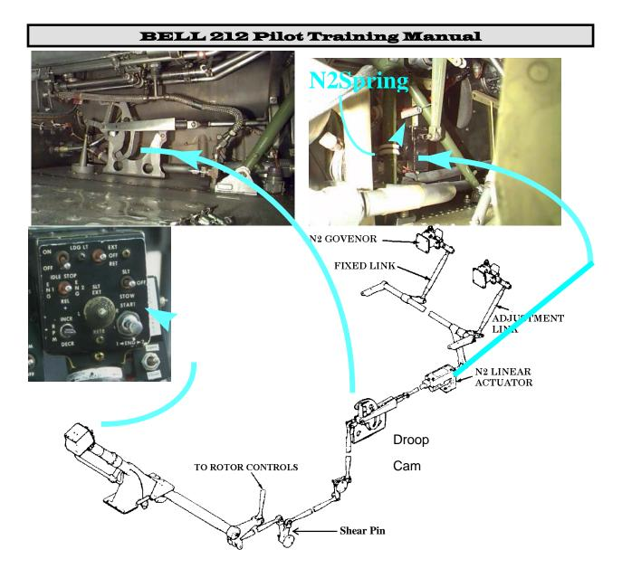
Figure 7-40 RPM Beep Switch and Droop Compensator
