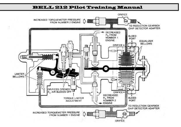
Figure 7-44 Torque Limiting
